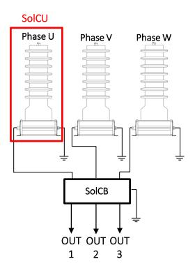
The SolPDOnline system is equipped with three Coupling Units and a connection box with three outputs.
