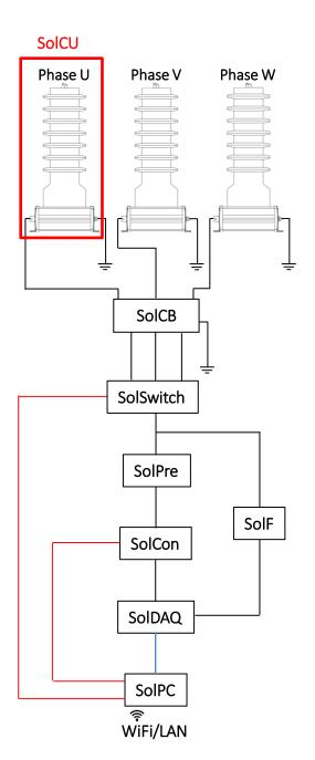
SolPDOnlinePlus allows continuous remote monitoring of partial discharge signals in the absence of an operator.
