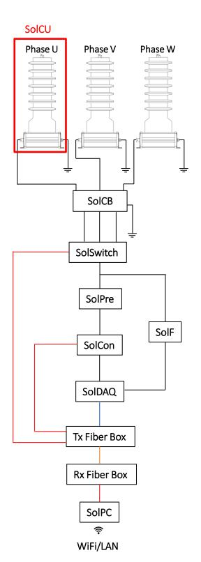
SolPDOnlineFiber allows continuous remote monitoring of the partial discharge signals coming out of SolCB in the absence of an operator.
